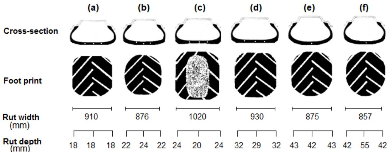
Figure 4. Mechanistic model of cross-section and footprint, rut width and depth of soil-tire interface for different loads and inflation pressures: (a) 31 load, tire inflation pressure of 50 kPa, (b) 31 load, tire inflation pressure of 100 kPa (c) 71 kN load, underinflated inflation pressure of 50 kPa; and (d) 71 kN load, correct inflation pressure of 100 kPa, (e) 71 kN load, overinflated pressure of 200 kPa; (f) 71 kN load, overinflated pressure of 300 kPa.
