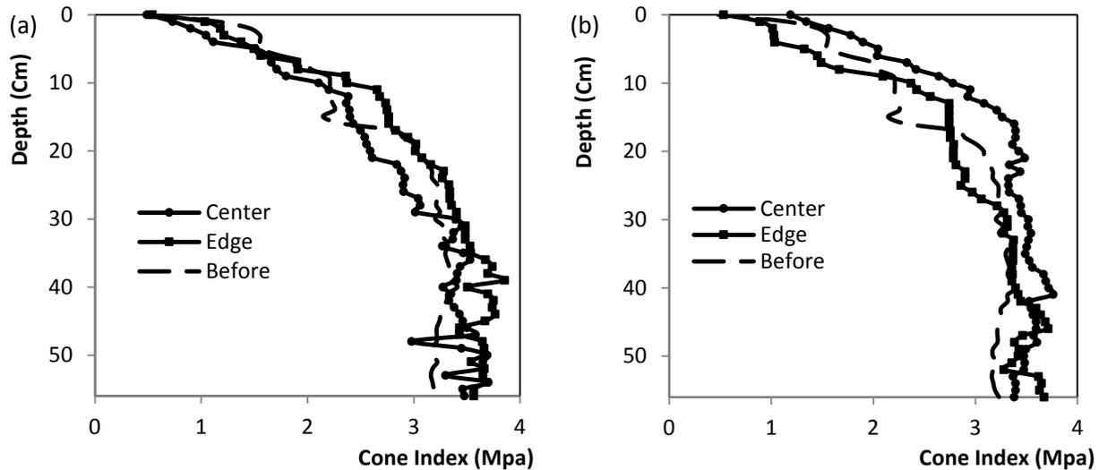
Figure 7. Cone index as measured in the track of a Alliance 30.5LR32 flotation tire: (a) 56.93 kN load, tire inflation pressure of 200 kPa; and (b) 56.93 kN load, tire inflation pressure of 300 kPa.
