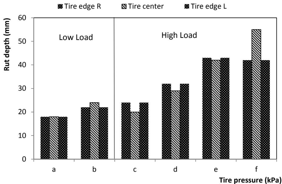
Figure 5. Rut depth of a 850/50 R30.5 tire for different loads and inflation pressures: a) 31 load, tire inflation pressure of 50 kPa, b) 31 load, tire inflation pressure of 100 kPa, c) 71 kN load, underinflated inflation pressure of 50 kPa; and d) 71 kN load, correct inflation pressure of 100 kPa, e) 71 kN load, overinflated pressure of 200 kPa; f) 71 kN load, overinflated pressure of 300 kPa.
