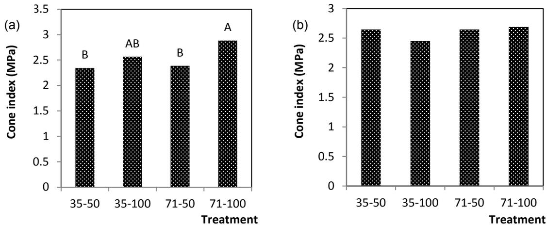
Figure 3. Interaction results for cone index (a) at the center and (b) at the edge of the tire track
