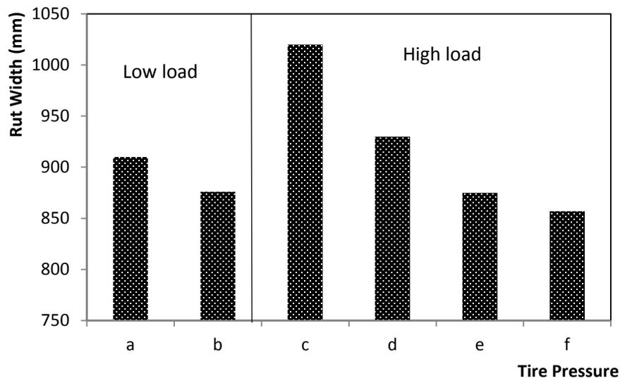
Figure 6. Rut width of a 850/50 R30.5 tire for different loads and inflation pressures: (a) 31 load, tire inflation pressure of 50 kPa, (b) 31 load, tire inflation pressure of 100 kPa (c) 71 kN load, underinflated inflation pressure of 50 kPa; and (d) 71 kN load, correct inflation pressure of 100 kPa, (e) 71 kN load, overinflated pressure of 200 kPa; (f) 71 kN load, overinflated pressure of 300 kPa.
