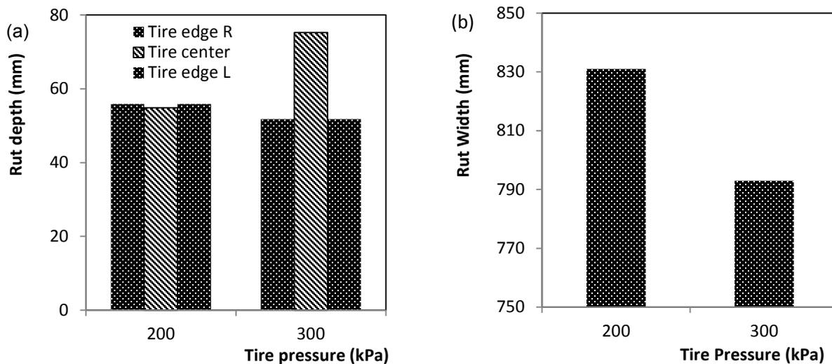
Figure 8. Rut depth and width under 56.93 kN load and tire pressures of 200 and 300 kPa.
