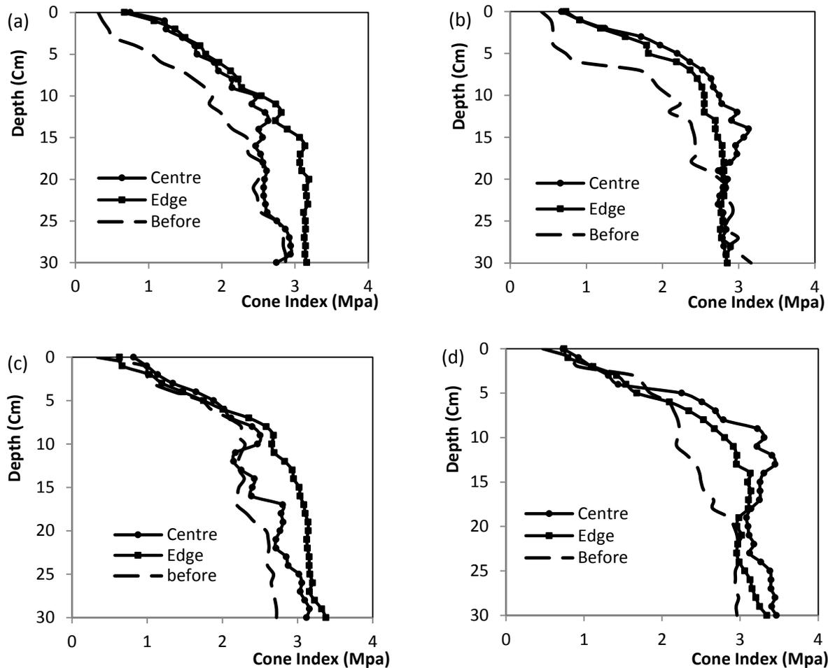
Figure 2. Cone index as measured in the track of a 850/50 R30.5 tire: (a) 35 kN load, tire inflation pressure of 50 kPa; (b) 35 kN load, tire inflation pressure of 100 kPa; (c) 70 kN load, tire inflation pressure of 50 kPa; and (d) 70 kN load, tire inflation pressure of 100 kPa.
